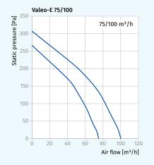
• The abrupt curves show high pressure performance and constant air flow of several **Valeo-E** fans integrated into a single ventilation shaft.
