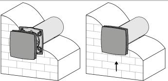
7. Install the outer ventilation hood or the grille.
