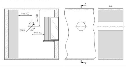
2. Install the air duct into the hole so that its cuts are aligned with the outside and inside surface of the wall. For ease of installation use the foam wedges included in the delivery.
